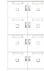
TLL168DR8/LB 1680h x 800w x 473d TLL169DR8/LB 1680h x 900w x 473d TLL161DR8/LB 1680h x 1000w x 473d
