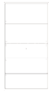
TLF1783D32F4 1780h x 800w x 473d TLF1793D32F4 1780h x 900w x 473d TLF1713D32F4 1780h x 1000w x 473d TLF17113D32F4 1780h x 1100w x 473d
